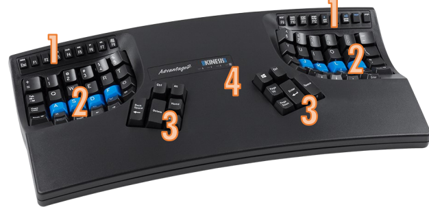
Fig 1. Advantage2 keyboard showing geometry and key groupings
