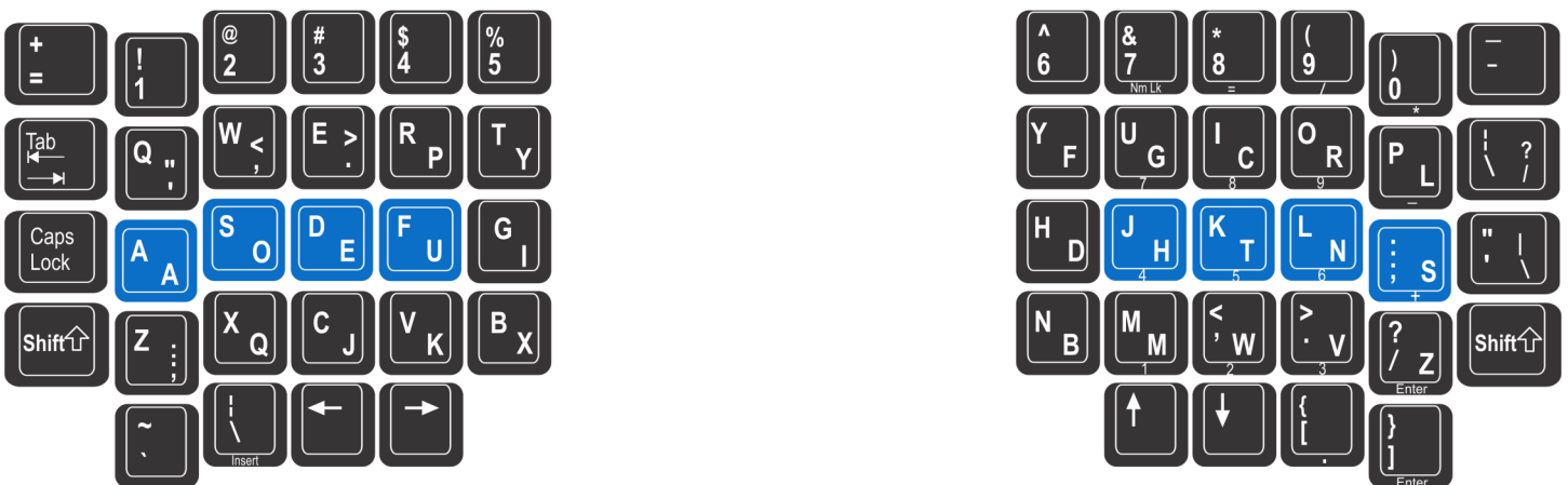
Fig 13. QWERTY-Dvorak dual-legged keycaps for Advantage2
